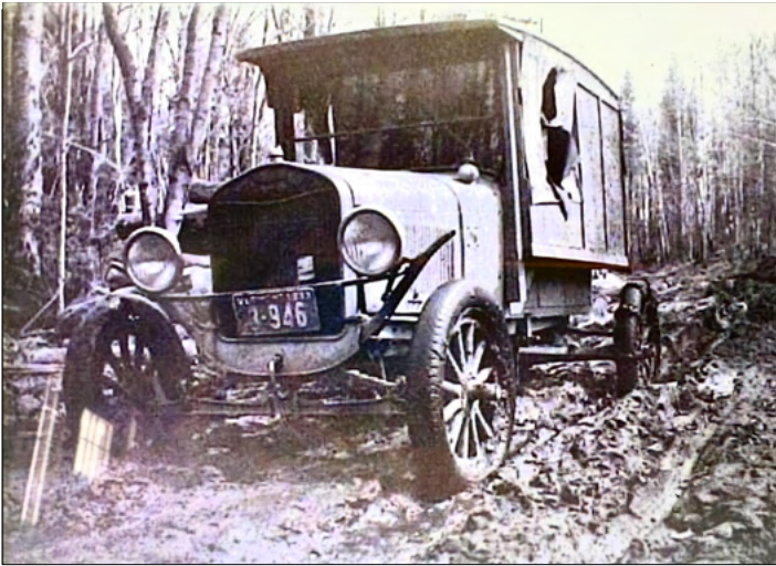
Jim Benzie modified his 1915 Model T Ford to carry the mail and equipped it with Page chains for both winter and mud season use. He also purchased a Snow Flyer Conversion Kit so he no longer had to use the horse and sleigh in the winter and could rely just on the Model T.
